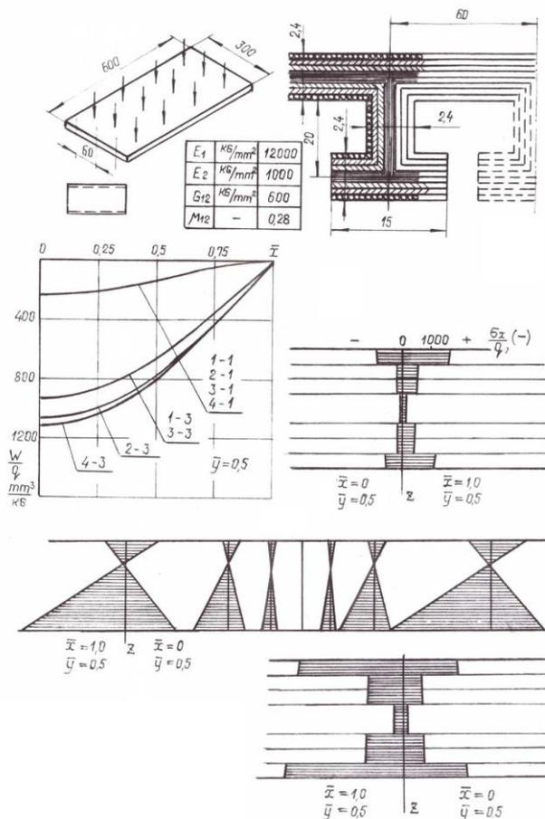
**Figure 1.** The panel, stiffened in longitudinal direction.
