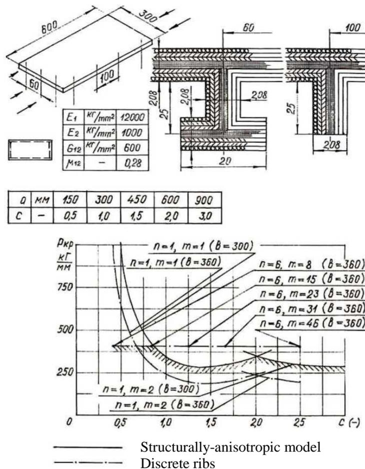
**Figure 3.** The panel with longitudinally-lateral stiffening set.
