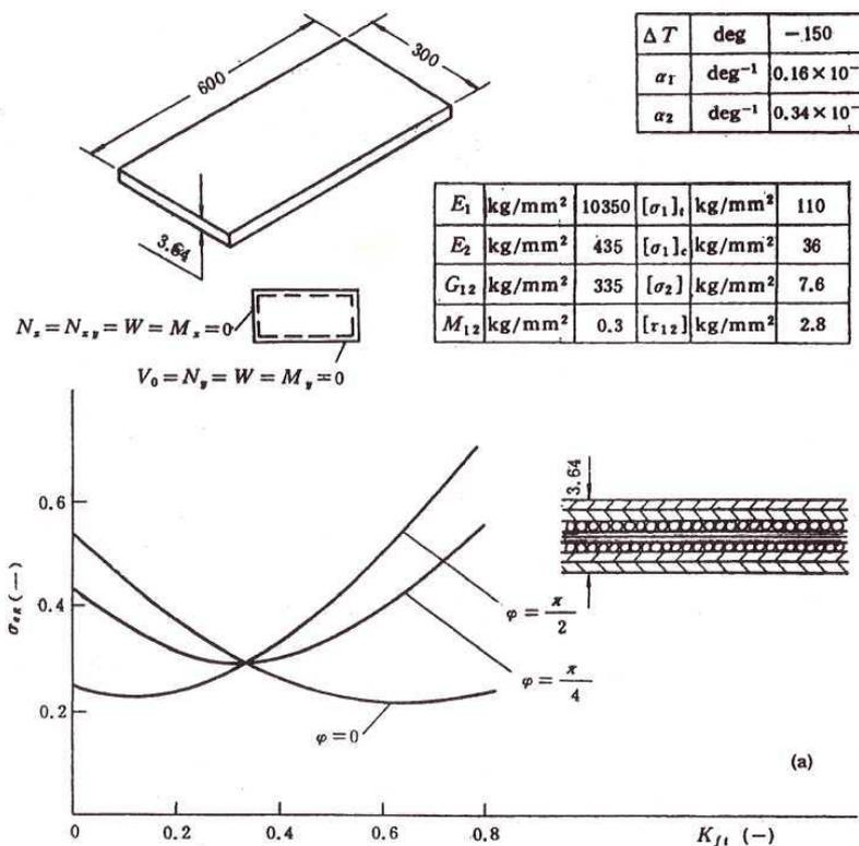
**Figure 2.** The panel with non-symmetric package structure. The influence of the reinforcing fibers preliminary tension on the residual temperature stresses
