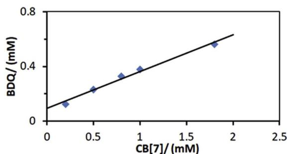
Fig. 3. Phase solubility diagram of BDQ in the presence of increasing concentrations of CB[7] (0.2, 0.5, 0.8, 1.0, 1.6 and 2.0 mM), determined from HPLC-UV chromatogram integrations (the linear fit equation:  $y = 0.270x + 0.093$ ,  $R^2 = 0.987$ ).
