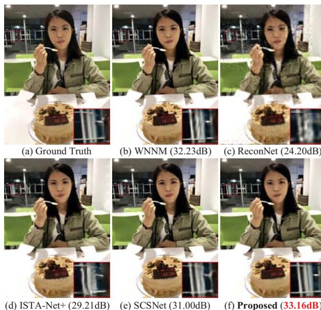
**Fig. 1.** CS results produced by our proposed H-PnP and state-of-the-art algorithms, when the CS ratio is 10%. (a) The original image; (b) WNNM [6]; (c) ReconNet [7]; (d) ISTA-Net<sup>+</sup> [3]; (e) SCSNet [8]; (f) the restored image by our proposed H-PnP, where the ringing artifacts have been eliminated significantly and sharp details are recovered.
